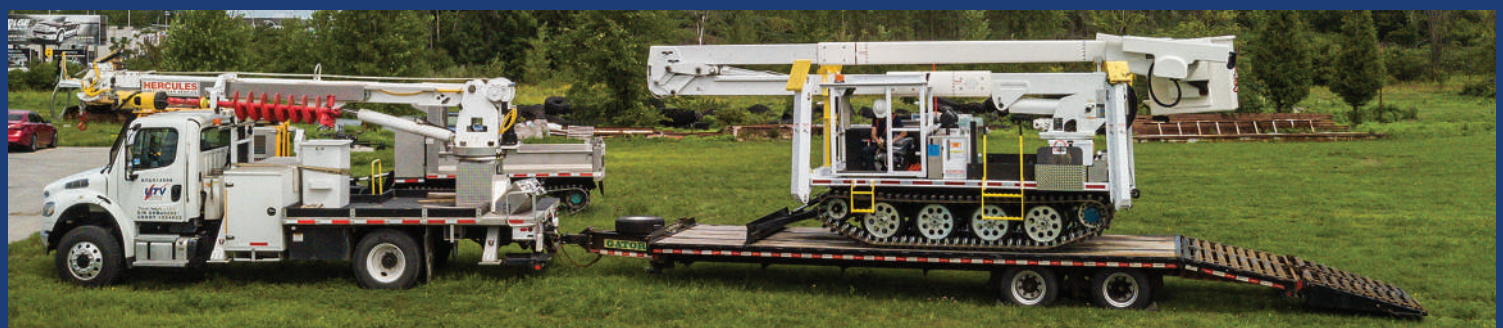
UTV Achiever Carrier with a Terex Optima TC-55 High Ranger
