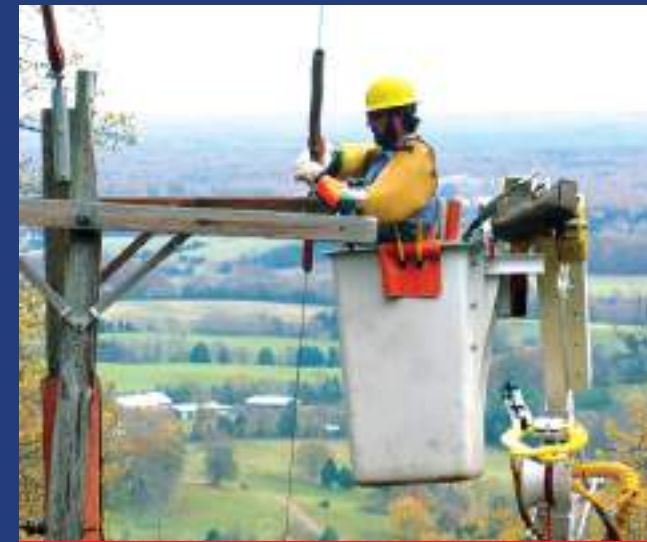
The insulated bucket has a 47' reach and comes with full pressure controls and an optional tool outlet and jib
