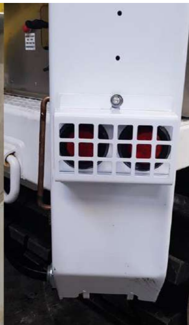
Rear Outriggers: Red Clearance & Turn Signal Lights
