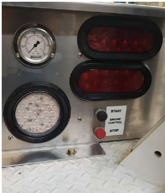
Rear Stop/Turn/Tail Lights, Reverse Lights Both Sides
