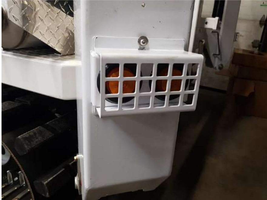
Front Outriggers: Amber Clearance & Turn Signal Lights
